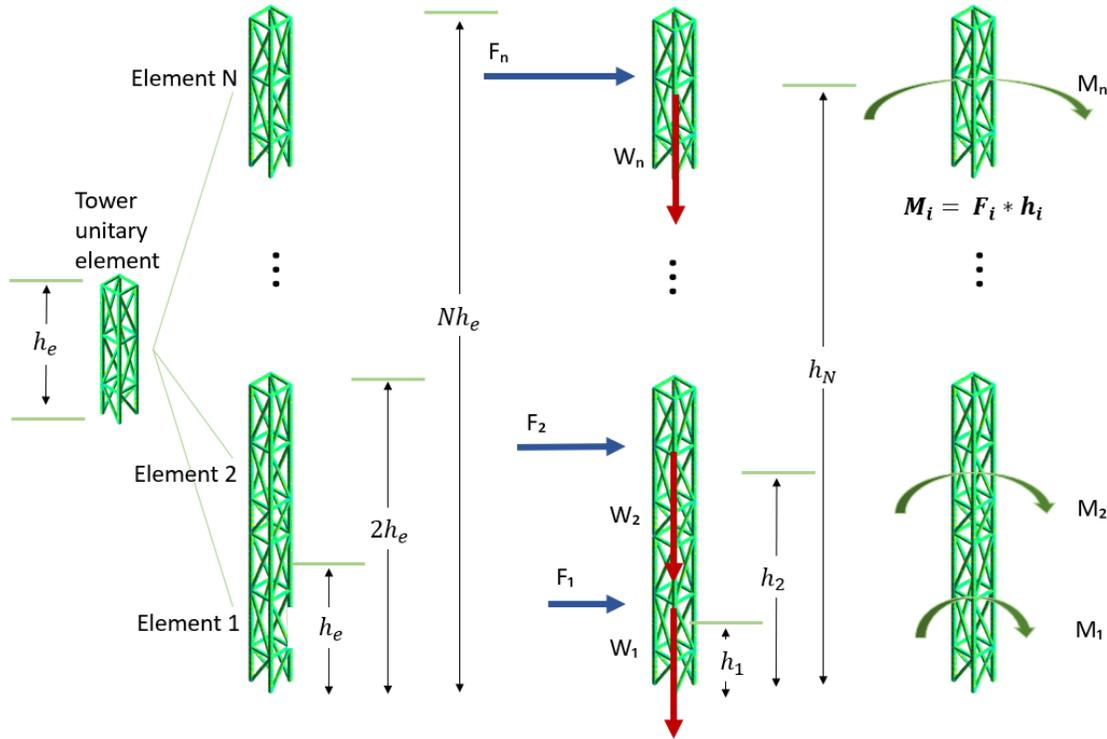
**Figure (2):** Modelling of the tower loads.
