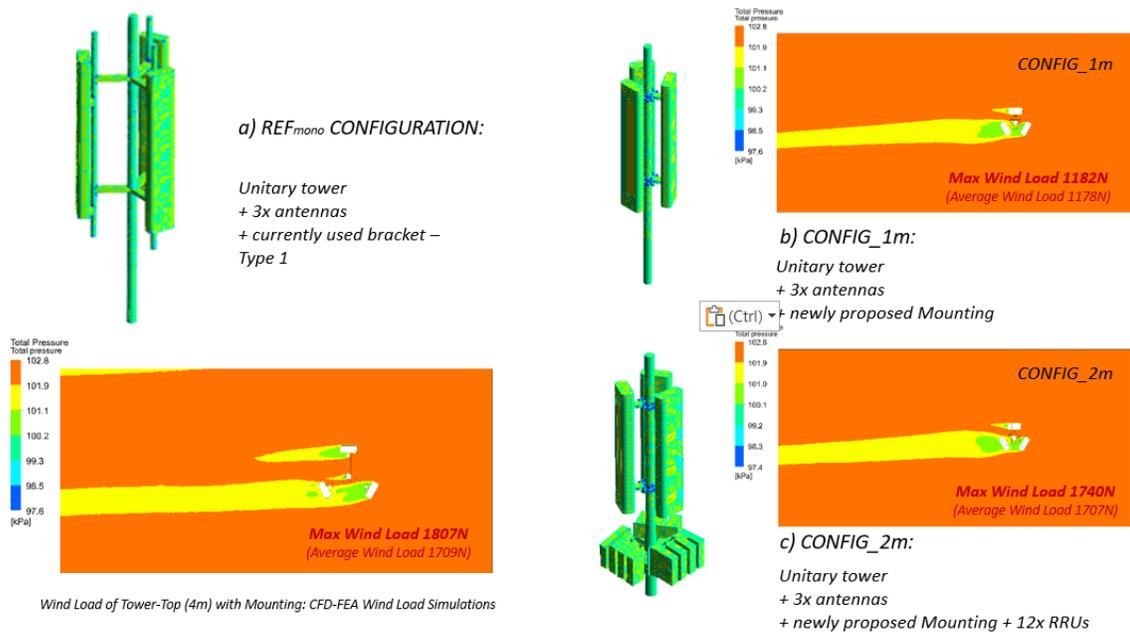
**Figure (5):** Wind pressure acting on monopole segment. (a) REF<sub>mono</sub>, (b) CONFIG\_1m, (c) CONFIG\_2m.
