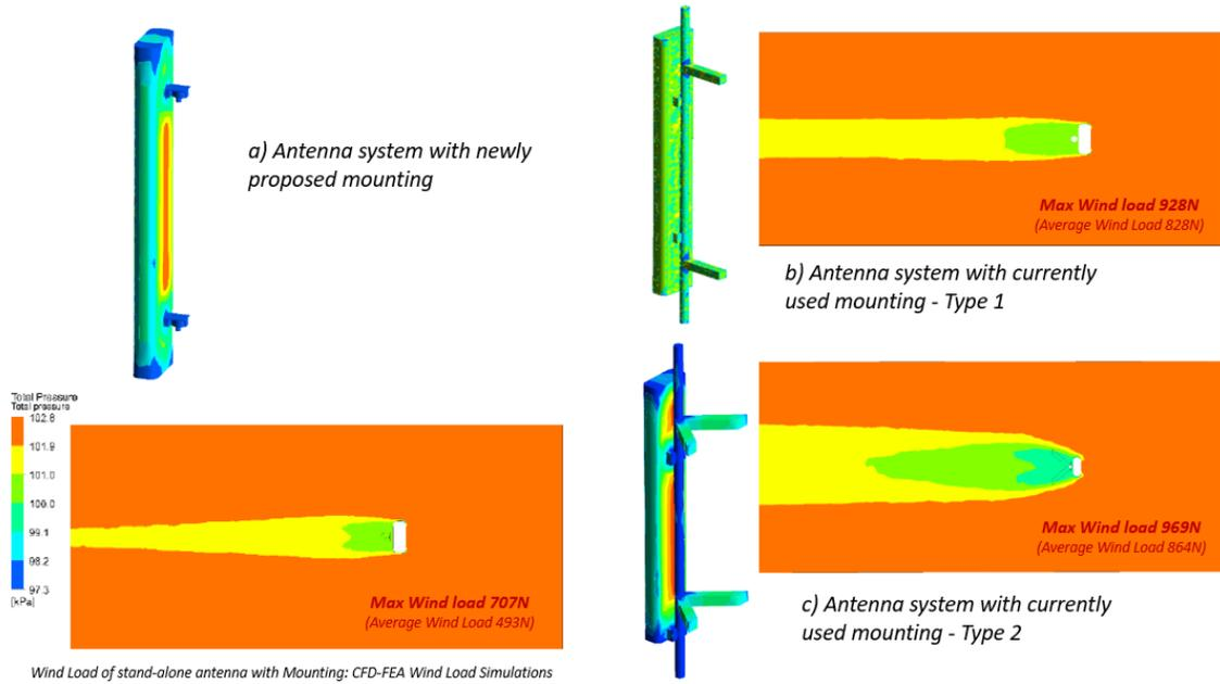
**Figure (3):** Wind pressure acting on standalone antenna and (a) the newly proposed bracket, (b) currently in use bracket - Type 1, (c) currently in use bracket - Type 2.
