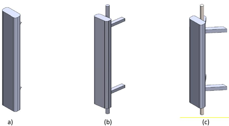
**Figure (1):** CAD models of antenna – bracket systems used throughout the present study. (a) antenna with the newly proposed bracket, (b) antenna with currently in use bracket - Type 1, (c) antenna with currently in use bracket - Type 2.
