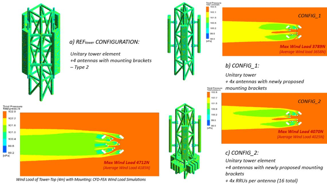
**Figure (4):** Wind pressure acting on lattice segment. (a) REF<sub>tower</sub>, (b) CONFIG\_1, (c) CONFIG\_2.
